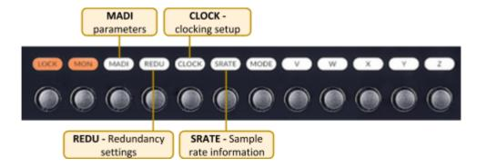
The Options menus are accessed by individual buttons to instantly navigate to the desired settings page on the OLED Display. The front panel must be unlocked for these buttons to function.
