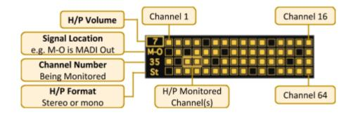
By default when entering the monitoring page the encoder will adjust the headphone volume. Pressing the **SELECT** encoder will move the focus to alter **Signal Location**. The options are:
